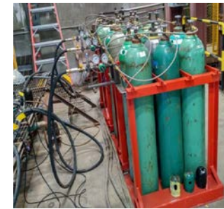
Fig 2. Left: Three sets of six bottles that supply flow through the sections of the receiver. Right: Bladed receiver flow path.
